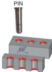
Chamfer with 60° used for deburring before "pin". 60° chamfer is easier than 90° or 120° to locate the pin.
